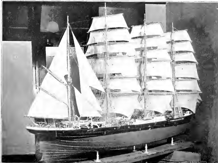
A beautiful model of the four-masted steel bark Pamir, constructed with all details on a scale of one-quarter inch to the foot, in the shops of the Museum of Science and Industry, Chicago.
